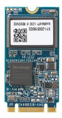
Nextorage A1 Series is a SATA SSD which comes with extremely reliable PLP (Power Loss Protection) technology and wide-range operation temperature. It is suitable for control units of embedded systems, edge computing, boot drive, data storage and much more.
