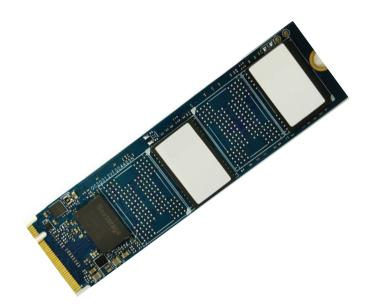
Nextorage E3 Series is a PCIe SSD which comes with extremely reliable PLP (Power Loss Protection) technology and supports high-speed interface. E3 Series is mainly designed for industrial use. It is suitable for control units of embedded systems, edge computing, boot drive, data storage and much more.
