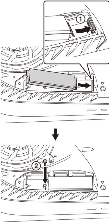
6. Insert the end of the M.2 SSD expansion slot cover into the PS5 (①), and then align the cover with the screw hole, hold it in place, and fasten it with the screw you removed in step 2 (②).
