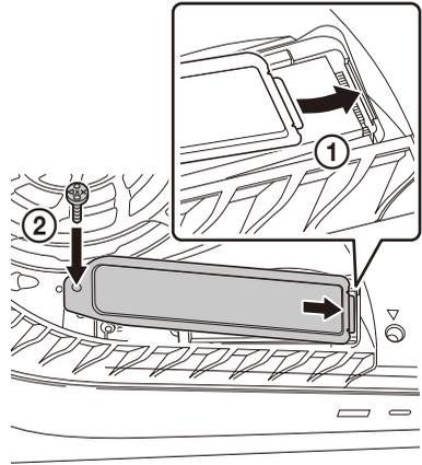
7. Attach the PS5 panel. Align the hooks on the panel with the attachment positions on the PS5, and then slide the panel to attach it.
