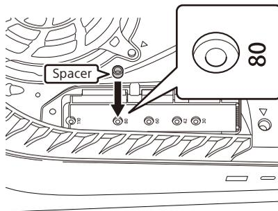
5. Taking care that the spacer does not move, insert the SSD into the M.2 SSD expansion slot connector (①) and then align the end opposite to the connector with the screw hole, hold it in place, and secure it with the screw you removed in step 3 (②). Overtightening the screw may damage the SSD or M.2 SSD expansion slot.
