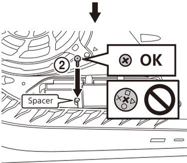
6. Insert the end of the M.2 SSD expansion slot cover into the PS5 (③), and then align the cover with the screw hole, hold it in place, and fasten it with the screw you removed in step 2 (④).
