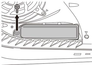
3. Remove the M.2 SSD mounting screw and spacer attached to the PS5.
