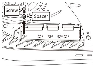
4. Place the spacer you removed in step 3 into the screw hole marked "80".
